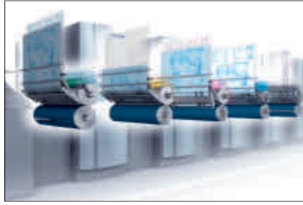
Staggered plate changes with AutoPlate Pro – quick, easy, and fully automatic.
