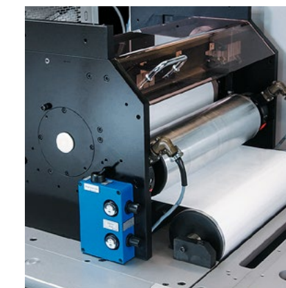
State-of-the-art servo drive technology for the printing cylinder and web feed system ensures optimum cost-effectiveness and substrate flexibility.
