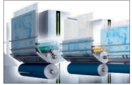
Staggered plate changes with AutoPlate Pro – quick, easy, and fully automatic.
