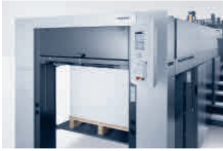
Uninterrupted production with the automatic non-stop system at the delivery.
