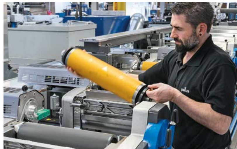
The newly developed flexographic printing unit of the Gallus Labelmaster supports extremely fast cylinder changes, enabling job changes within seconds.
