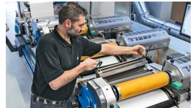
The ink chamber can be easily changed in just a few quick steps.
