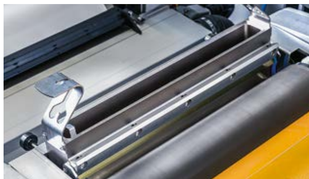
The ink chamber is also designed for high printing speeds, thus reducing foaming and ensuring optimum ink transfer to the anilox rollers.
