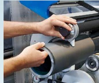
Frontloading anilox sleeve permits quick and easy exchange.
