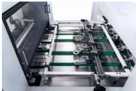
The feed table is equipped with two central suction belts for stable and secure sheet transport. It features ultrasonic double sheet controls. Before arriving at the front-lays, the sheets are slowed down.
