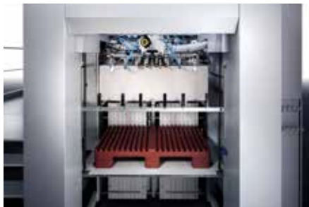
The machine is equipped with a manual non-stop feeder and a suction head with quick adjustment.
