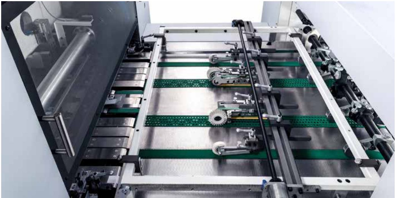
TOP: Feed Table with suction belts and hand wheel for central adjustment of the rollers and brushes
