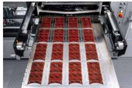
The Promatrix works with a 4+1mm cutting plate system (4mm thick cutting plate plus 1mm thin cutting plate). Pneumatic unlocking/locking is standard – as is air support for pulling out the cutting plate.
