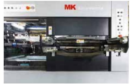
The Easymatrix works with a 4+1mm cutting plate system (4mm thick cutting plate plus 1mm thin cutting plate). An optional 5mm cutting plate is also available.
