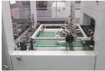
The feed table with eight transport belts and a hand wheel for central adjustment of rollers & brushes. Before arrival at the front-lays, the sheets are slowed down.
