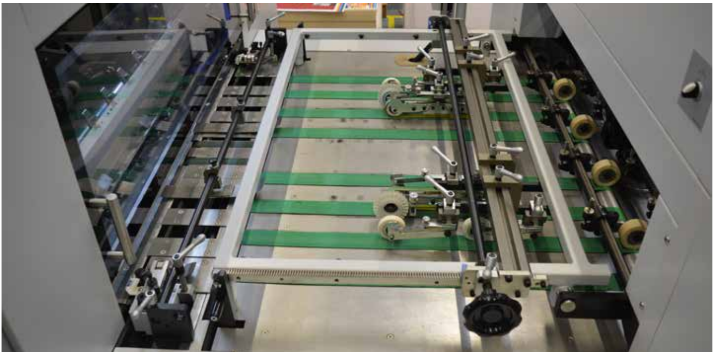
TOP: Feed table with eight transport belts and hand wheel for central adjustment of rollers and brushes.
